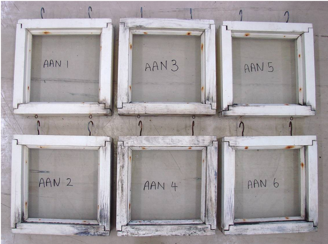
E. delegatensis = Alpine ash (AAN) – azole LOSP using a commercial schedule, painted white.
