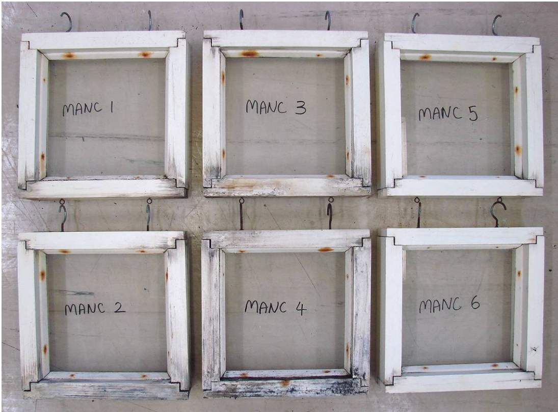
E. regnans = Mountain ash (MANC) – azole LOSP using a commercial schedule, painted white.
