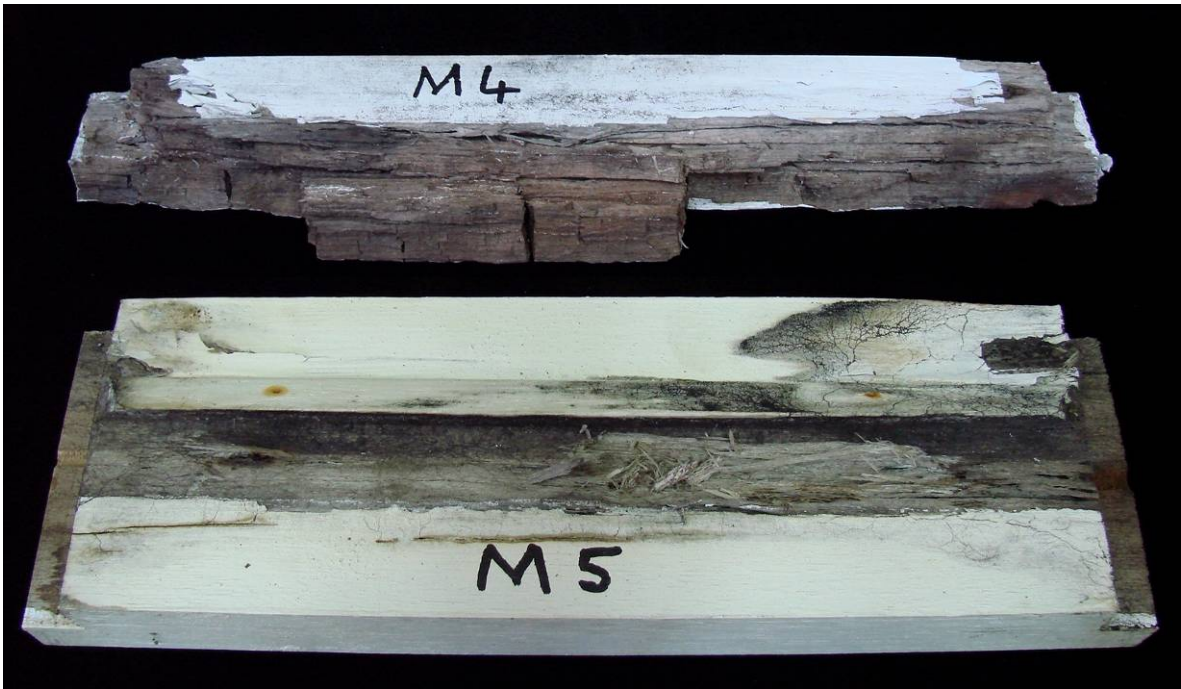
Figure 3. Bottom sills of untreated painted Shorea windows M4 (brown rot) and M5 (white rot) after eight years' exposure.
