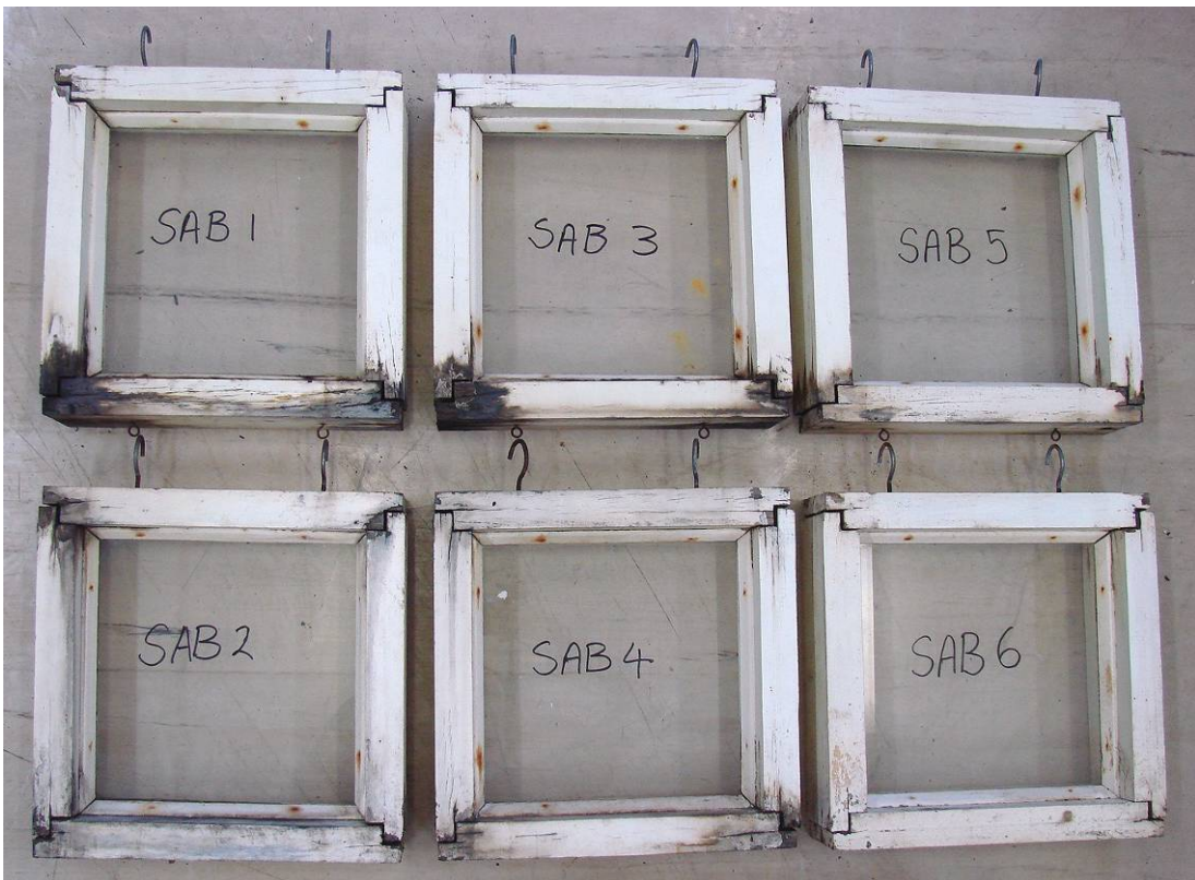
E. sieberi = Silvertop ash (SAB) – VPI boron treatment of green timber, painted white.
