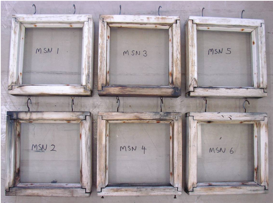
E. obliqua = messmate (MSN) – azole LOSP using a commercial schedule, painted white.
