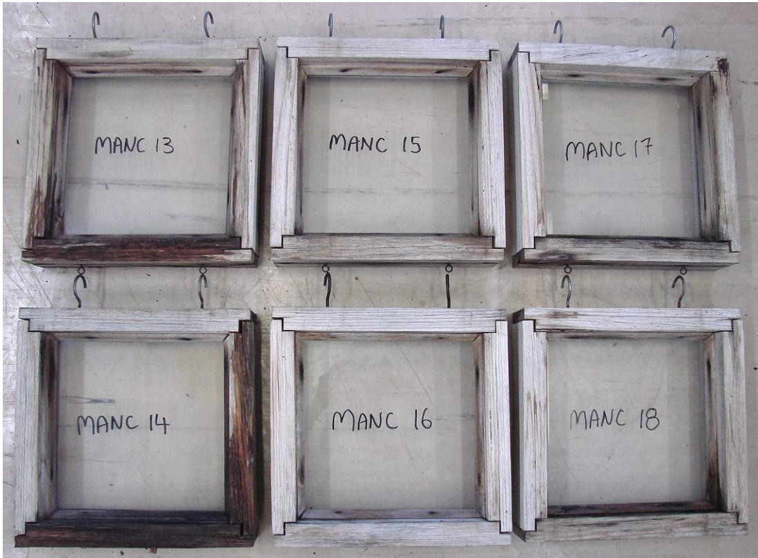
E. regnans = Mountain ash (MANC) – azole LOSP using a commercial schedule, unpainted.
