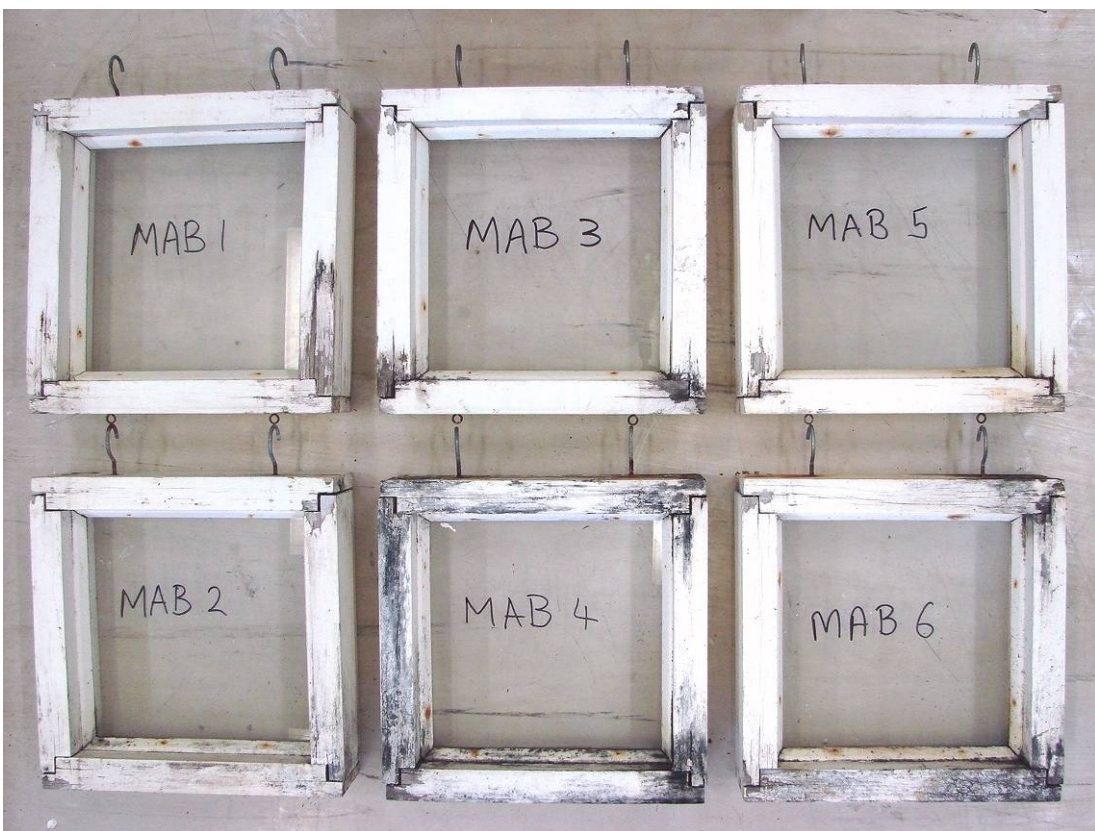
E. regnans = Mountain ash (MAB) – VPI boron treatment of green timber, painted white.
