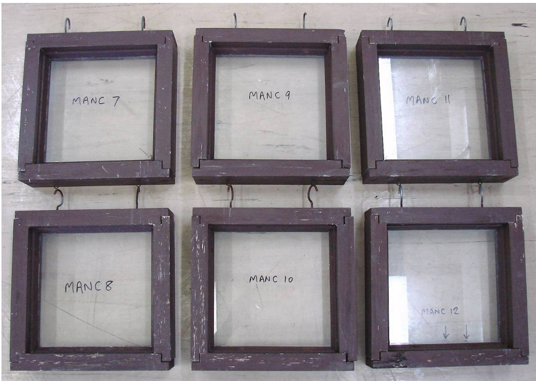
E. regnans = Mountain ash (MANC) – azole LOSP using a commercial schedule, painted white.
