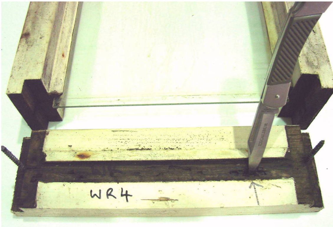
Figure 4. Bottom sill of untreated painted T. plicata window WR4 with 12 mm deep brown rot under glass + beading after eight years' exposure.
