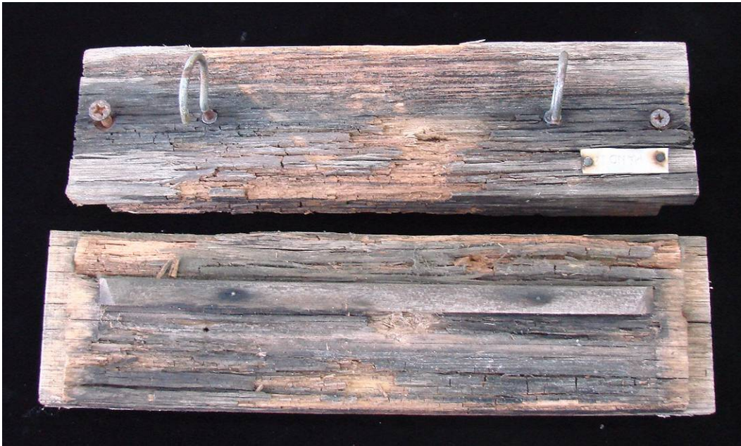
Figure 8. Unpainted azole LOSP-treated E. regnans windows. Top piece shows upper surface of top section of MAND14. Lower piece shows upper surface of bottom sill (one beading retained) of MAND13.
