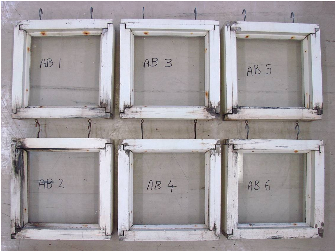
E. delegatensis = Alpine ash (AB) – VPI boron treatment of green timber, painted white.
