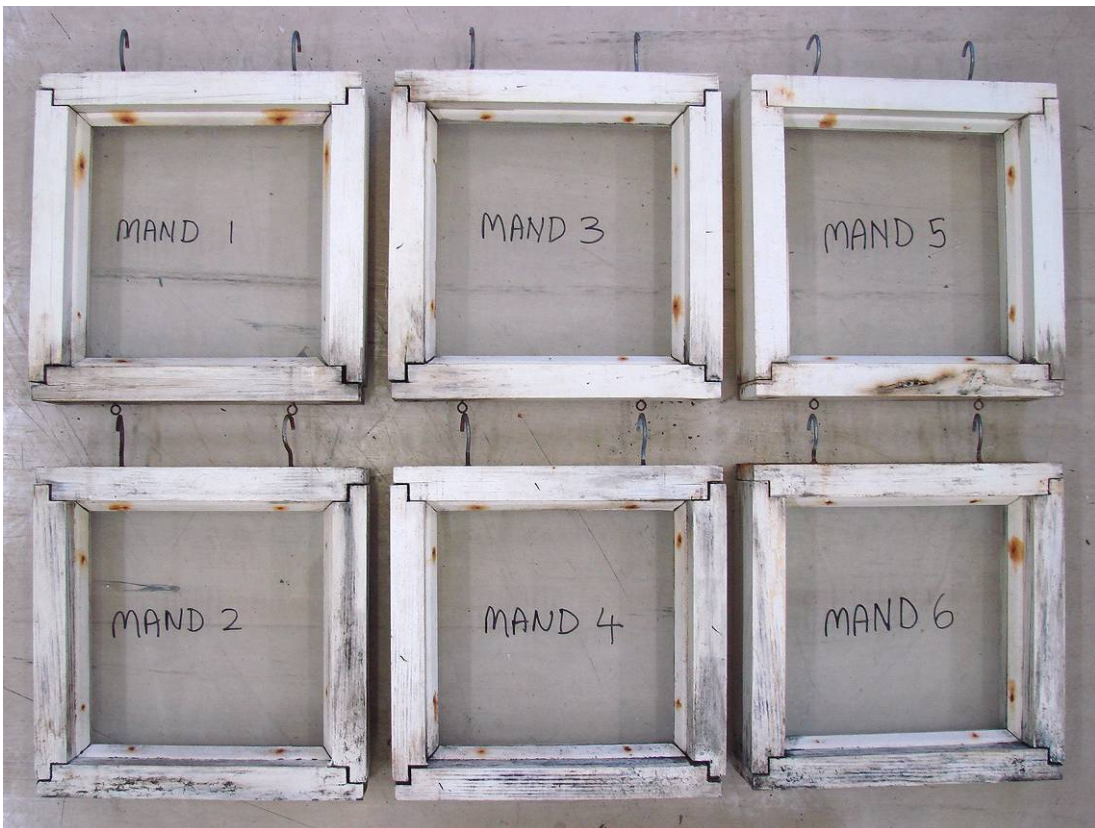
E. regnans = Mountain ash (MAND) – azole LOSP by 3 minute dip, painted white.
