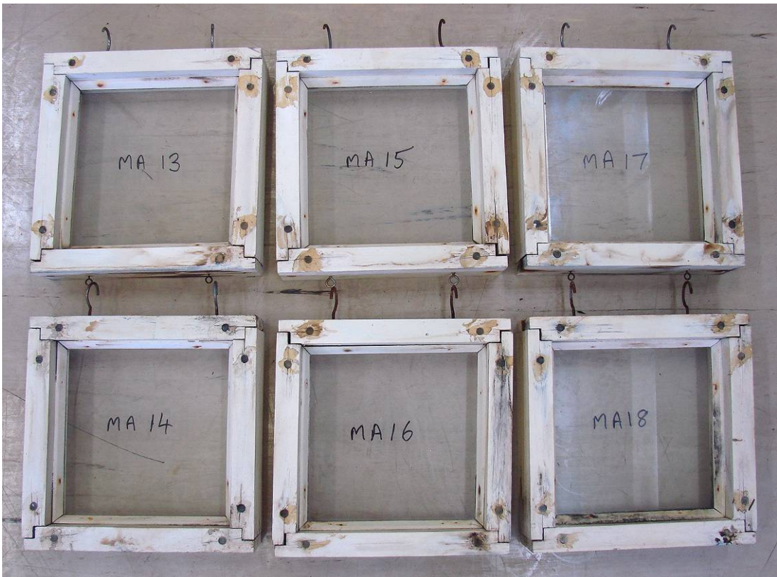
Untreated E. regnans = Mountain ash (MA) – but with No-rot rods, painted white. Note drill holes with rods near corners sealed with silicone.
