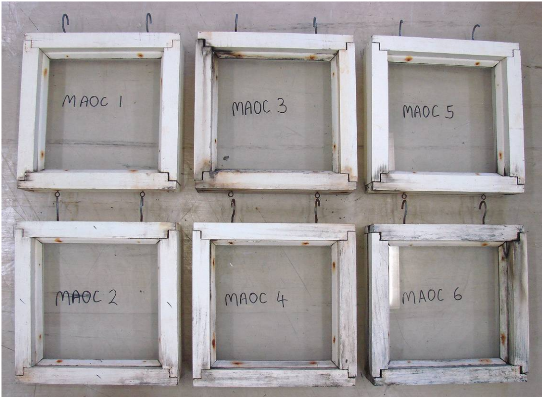
E. regnans = Mountain ash (MAOC) – TBTN LOSP using commercial schedule, painted white.
