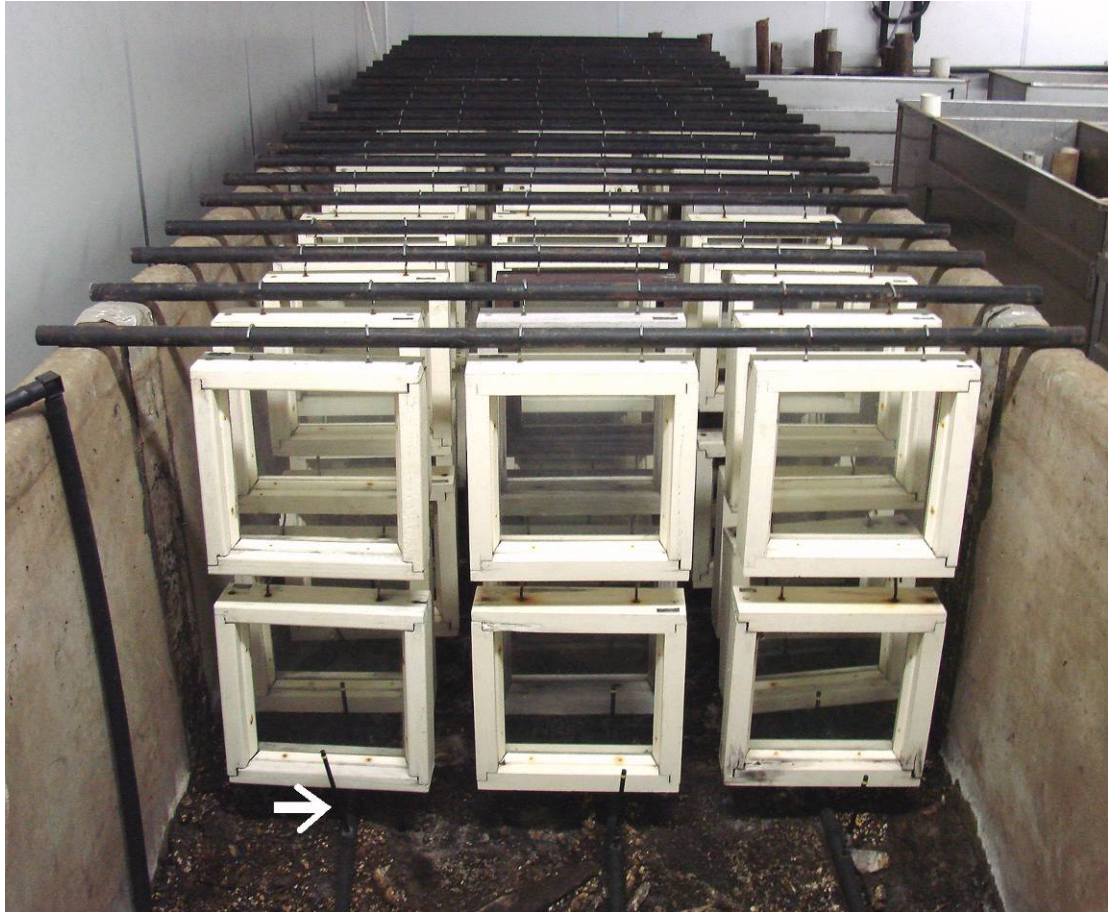
Figure 1. Exposure of model windows in the AFS. Note irrigation system (e.g. white arrow).
