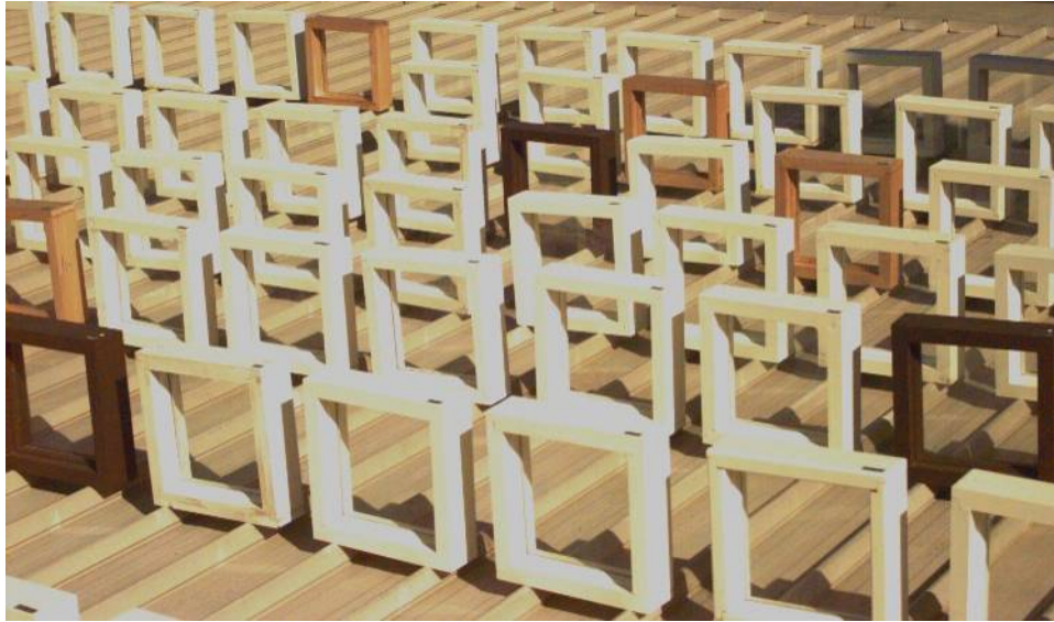
Figure 16. Summer exposure of model window frames on the roof of the Clayton laboratory.
