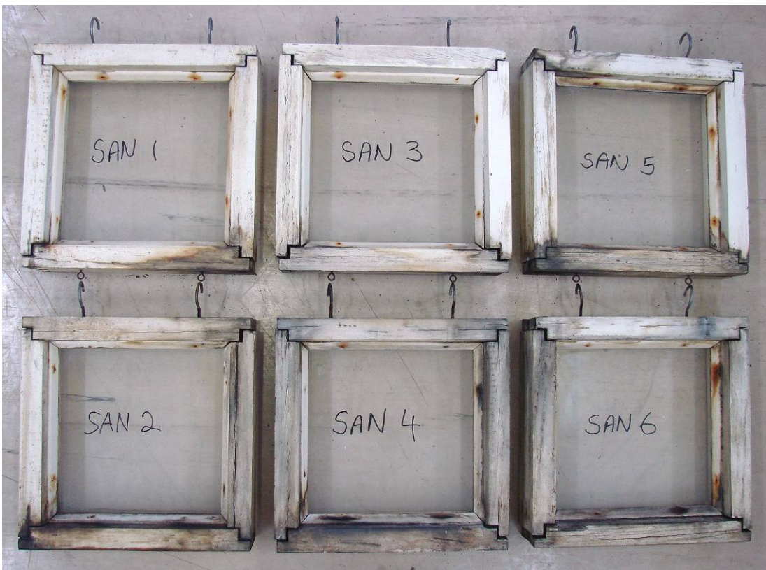
E. sieberi = Silvertop ash (SAN) – azole LOSP using a commercial schedule, painted white.
